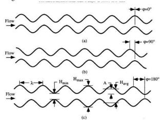
Figure 10: Schematic of wavy passage configurations and the definition of important geometric parameters "depth of channel is L"
