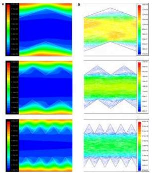
Figure 8: Variation of (a) temperature contour, (b) velocity vector for different channel heights at the same Re (918), wavy angle =  $40^{0}$ , q = 0.83 kW/m<sup>2</sup> [7]
