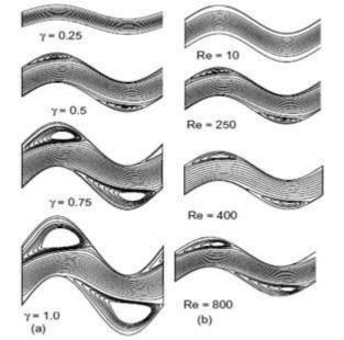
Figure 9: Streamline distributions in steady laminar flows in sinusoidal corrugated-plate channels [8]
