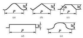
**Figure 5:** Corrugation profiles. (a) Sinusoidal curve, (b) triangular curve, (c) trapezoidal curve, (d) rectangular curve, and (e) elliptic curve. [5]
