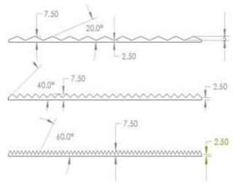
Figure 7: Schematic diagram of the corrugated plate. [7]
