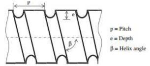
Figure 2: Drawing of a helically corrugated tube
