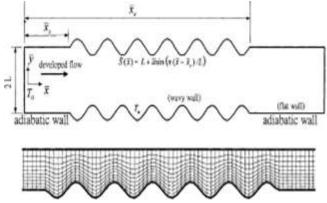
Figure 13: Physical model, coordinates and grid system [9]
