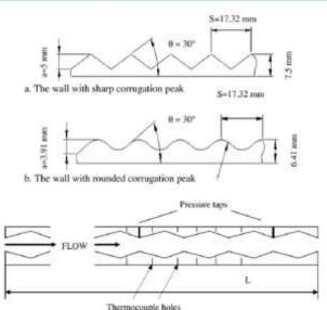
c. The temperature and pressure measurement points for the sharp-edge version of the corrugated duct used in the experiments.
