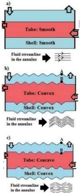
Figure 1: The effect of arrangement type on annulus fluid streamline [1]
