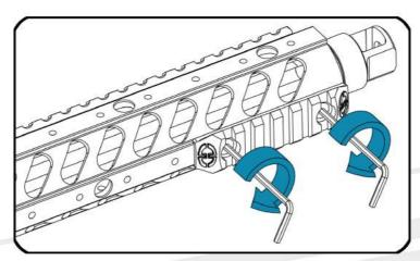
2 Secure the rail using two M4x10 screws from the screw set bag.
