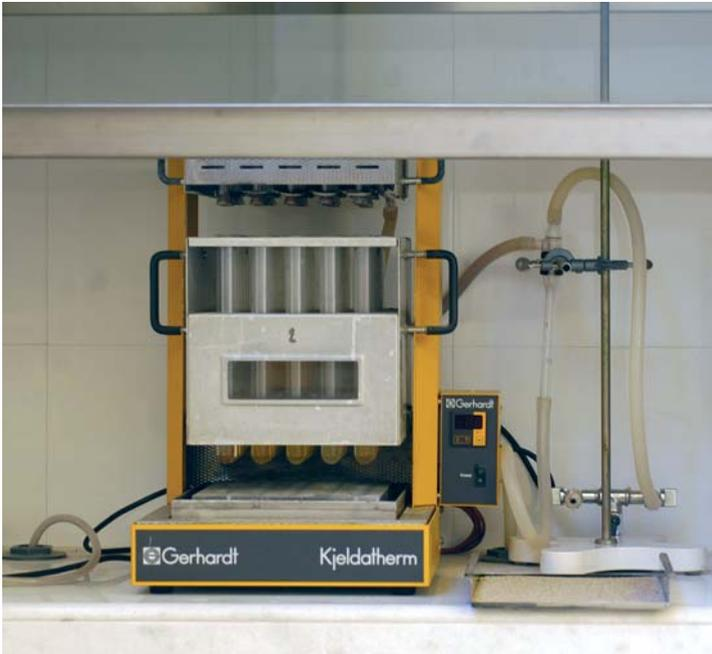
**Figura 4.3.** Digestor para Kjeldahl, modelo Kjeldatherm KB/KBL (Gerhardt Laboratory Systems, Alemania).
