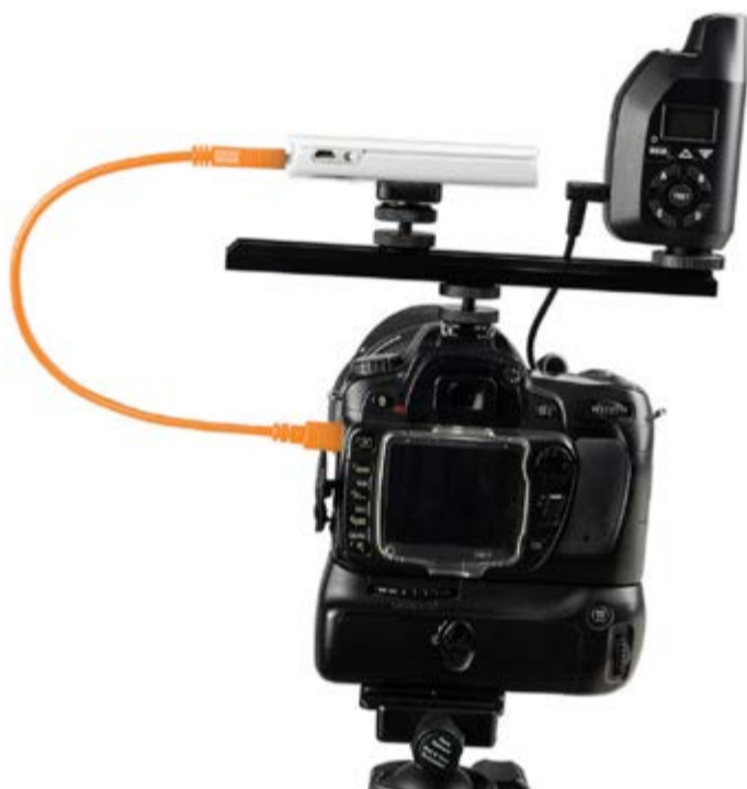
The CamRanger Wireless N transmitter connects to the camera through the USB port. It creates its own wireless connection between the camera and the phone, tablet or computer application that is receiving the images.
