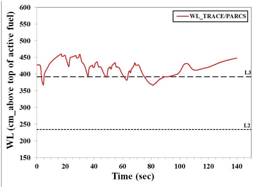
Figure 14 The water level (FMCRD run-in)
