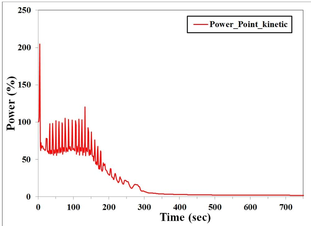
Figure 16 The core power (SLCS initiation)
