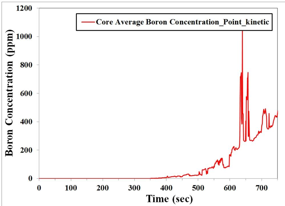
Figure 21 The core average boron concentration (SLCS initiation)
