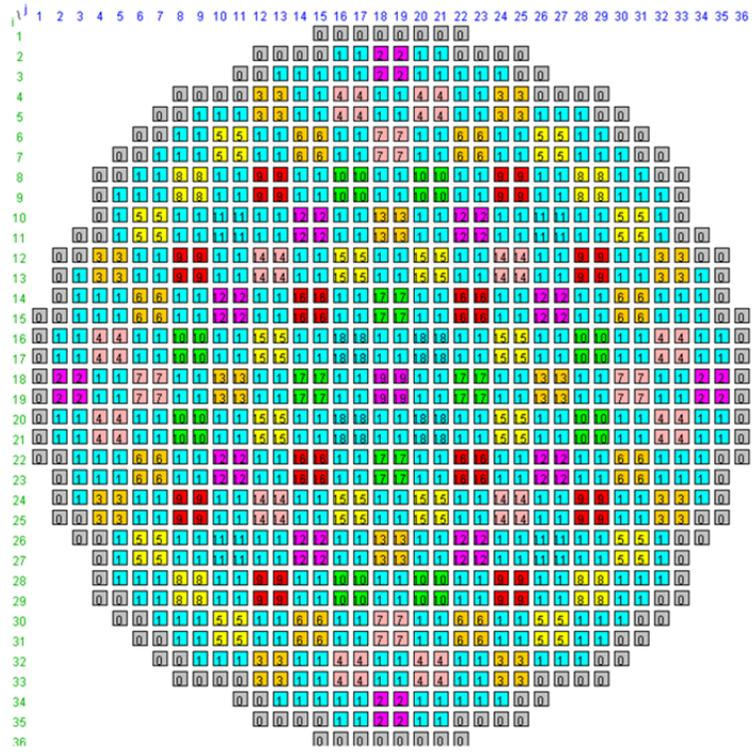
Figure 3 Control rod pattern for Lungmen PARCS model
