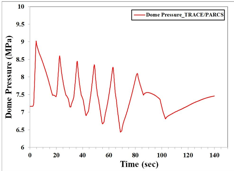
Figure 12 The dome pressure (FMCRD run-in)
