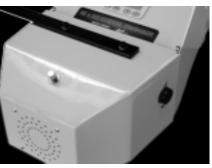
timer will reset to the preset time. BOTH black buttons must be pressed together, to insure that both operators hands are clear of the pressing area, for safety purposes.
