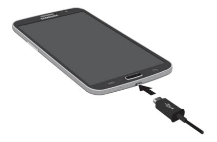
3. When charging is finished, remove the USB cable from the charger/accessory jack on the phone.
