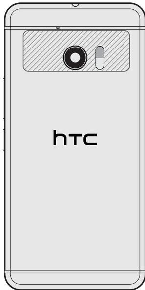
Make sure that the NFC area (shaded part) of HTC 10 and the other phone's NFC area are close to one another. Experiment by slightly moving the phones until a connection is made.
