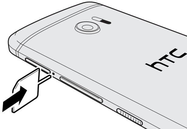
3. Push the tip all the way into the hole until the card tray ejects.
