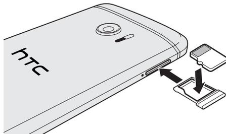
5. Insert the microSD card tray back into the slot.
