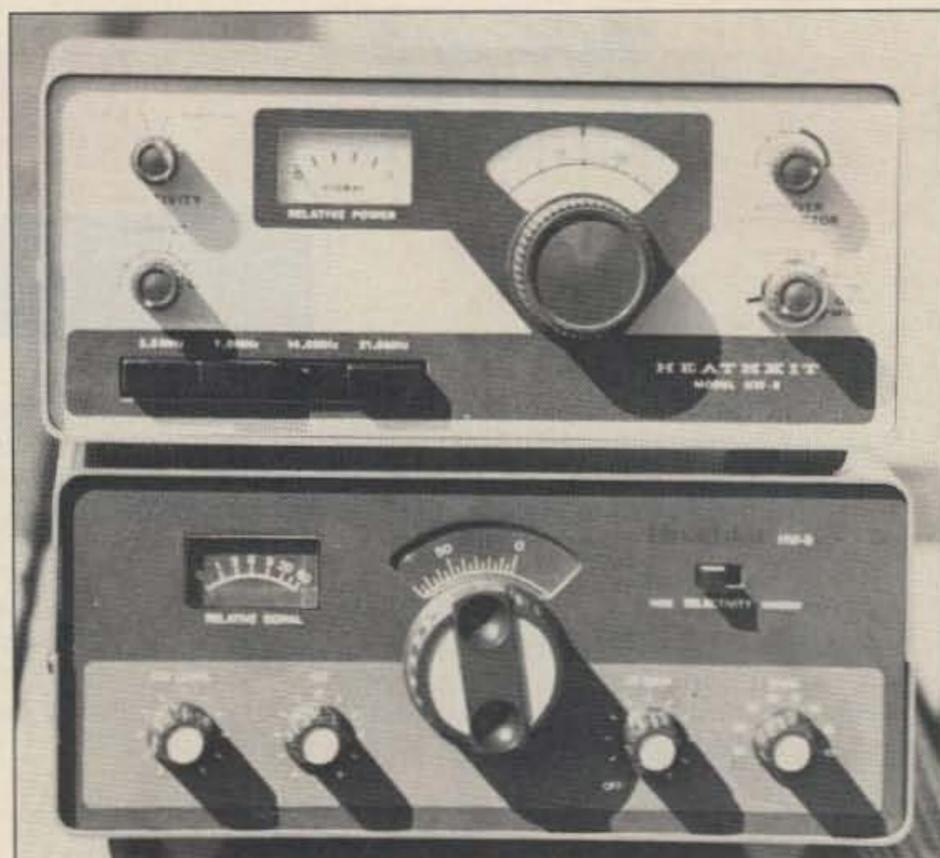
Photo A. The Heathkit HW-8 (top) and the HW-9 (bottom) QRP transceivers.
