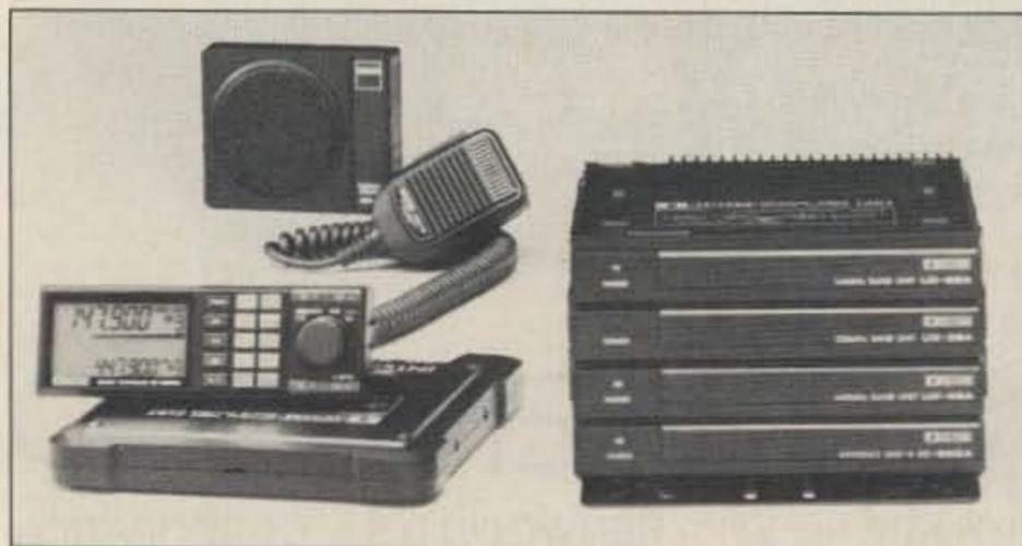
ICOM's IC-900 6-band mobile transceiver.
