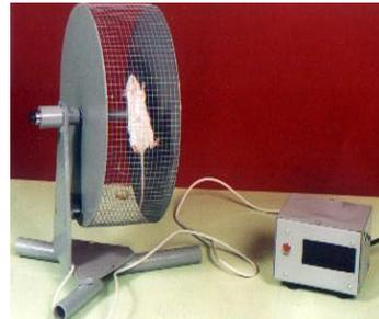
Gambar 2. alat ukur lokomotor hewan percobaan (*whell cage*)
