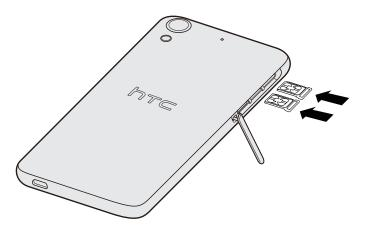
**6.** To close the slot cover, slide the plastic hinge into the side and press the cover until it clicks into place.
