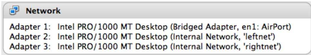
1. Set up two Linux machines, one on **leftnet**, the other on **rightnet**. Make sure they both get an ip-address in the correct subnet. These two machines will be 'left' and 'right' from the 'router'.
