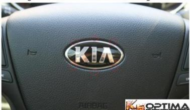
2. Start with your flat head screwdriver pushing down on the top three tabs. We recommend starting with the center tab. You want to push down towards the floorboard of the vehicle while simultaneously pulling the emblem/screwdriver towards you. This will take a bit of force and will slowly start to wiggle out.
