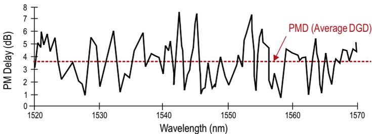
Figure 40: DGD as a function of optical wavelength
