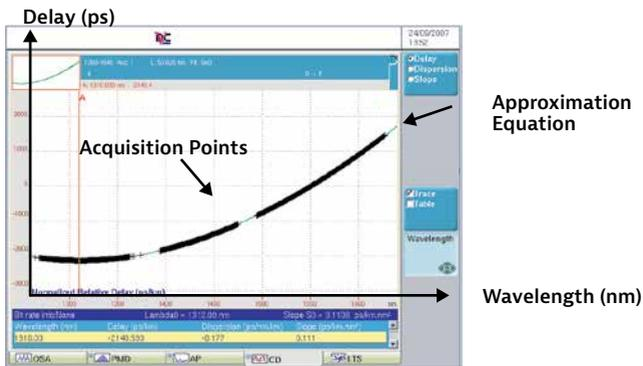
The CD is computed by calculating the slope of the group delay curve as a function of wavelength.
