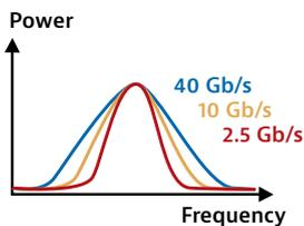
**Higher bit rate = less time between pulses**
