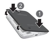
Press along the edge of the back cover (3) until you have a secure seal.
