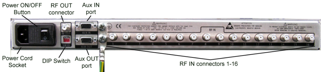
Figure 7 ISS RF Switch rear panel
